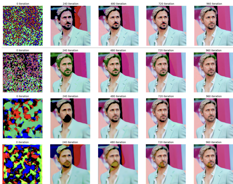
Figure 7. Denoising Results (Image 1 Architecture 1): First Row: Architecture 1, noise = 0.1, depth = 2. Second Row: Architecture 1, noise = 0.5, depth = 2. Third Row: Architecture 1, noise = 0.1, depth = 4. Fourth Row: Architecture 1, noise = 0.5, depth = 4
